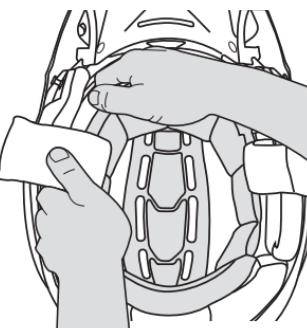
Gently pull cheek pads away from the interior wall of helmet to unsnap the plastic clips on each side.
