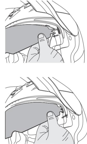
Firmly hold the sunvisor with your hand and gently pull one side out away from the helmet to release.
