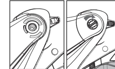
To install the side covers, first remove the peak visor. Then align each side cover over the faceshield side and with the peak visor screw hole.
