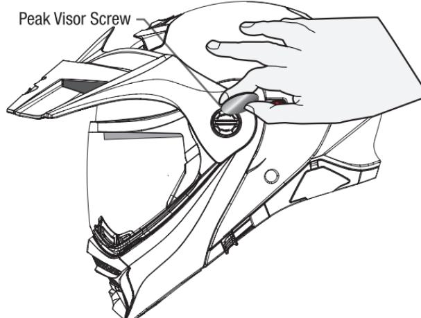
Once the new faceshield is in position, re-install the peak visor or side covers.
