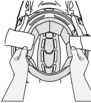
After removing the cheek pads, reach into the helmet and pull out the crown liner shown below. The front part of the liner is snapped to the helmet liner frame.
